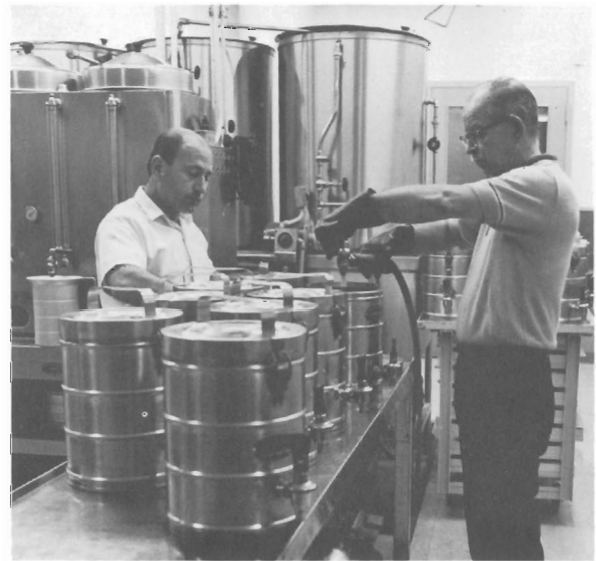
Piping-hot coffee from 90-gallon brewing vats is pumped into 1½-gallon pots for Palo Alto-Stanford area plants by Tony Pascual, left, and Ray Mierendorf. Quality is very carefully watched as is in-time distribution: Who wants 4,500 instant critics?
